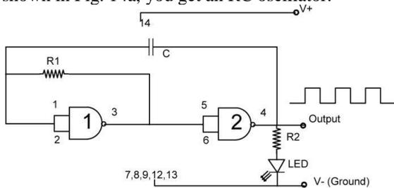
The output of NAND gate 2 will oscillate in a square wave form.
