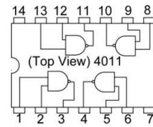
the operating Voltage range ( $V_{DD}$ ) is 3 to 15 Volts. We shall use the 6-volt supply of the MCC car.
