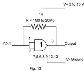
**How does it work?** The input and output will stabilise at half the voltage. Any change in input will be amplified as an output in the opposite direction. Lowering of the input will raise the output
