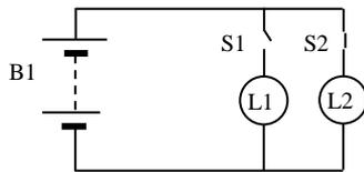
Volts. L1 is a car bulb rated at 12 Volts & 6 Watts. What is the resistance of the bulb when hot?
