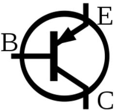
Diagram in the left is a PNP transistor. I have not shown an arrow in the C-B diode. As I said earlier, this is never drawn.
