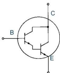
You can see how the 2 transistors are interconnected. When the transistor is on and saturated (when working as a switch), the Voltage between Base and emitter would be about 1.2 to 1.4 V as there are 2 transistors inside. The Collector-Emitter (C-E) volts
