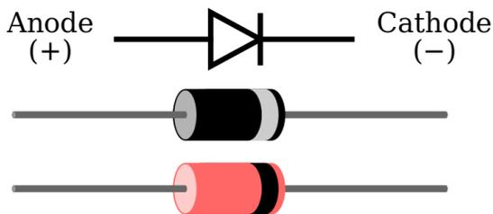
The current flows from the Anode to the Cathode. Note that the Cathode side has a band around it.
